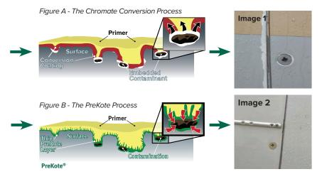
**About the photos to the right:** To compare the pretreatment process, a leading commercial airline treated one 737-800 with PreKote and another 737-800 with a chromate conversation coating. When the aircraft returned for a 24-month inspection, the airline declared PreKote provided superior protection and out-performed the chromate conversion coating.
